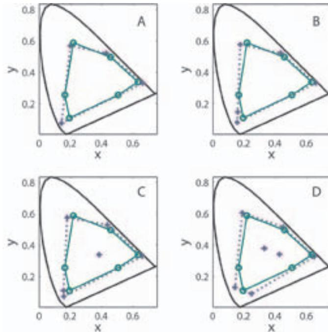
**FIGURE 5** — The chromaticity of the basis functions (dotted blue) compared to that of the solids C, M, Y, R, G, and B (solid green). A, B, C, and D are 4, 5, 6, and 7 basis functions, respectively.
