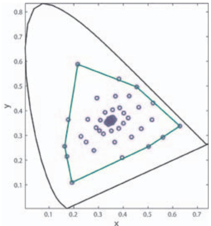
**FIGURE 2** — Chromaticity coordinates of 60 color patches printed on Matchprint proofing system. The green solid polygon defined by the solids spectra (CMYRGB) encloses all measured colors and defines the color gamut of the system.
