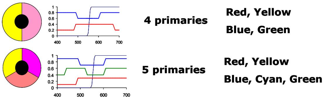
Figure 3. Schematics of dichroic mirror and color wheel spectral properties.
