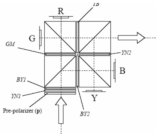
Figure 4. Schematics of ColorQuad based four-panel LCoS engine
