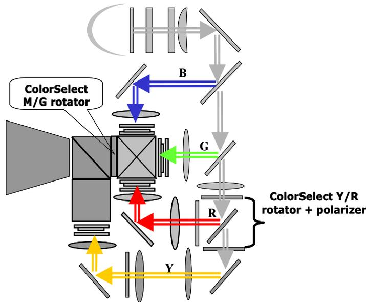
Figure 5. Schematics of the four-panel HTPS projector.
